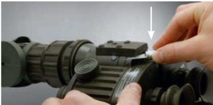
2. Remove the existing screws with a suitable tool, e.g. a small plier.
