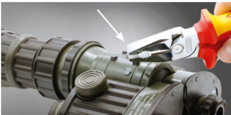
3. Mount adapter by screwing the large retaining screw as well as the and four additionally small 2.5mm screws.
